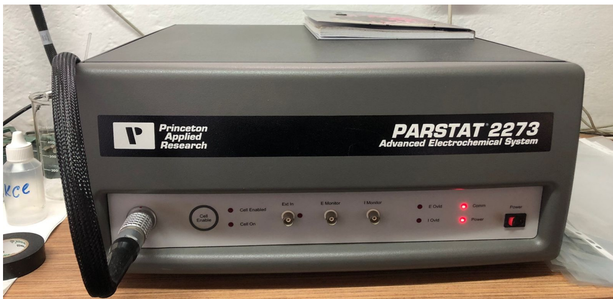
Slika 32. Potenciostat/galvanostat model Parstat 2273
