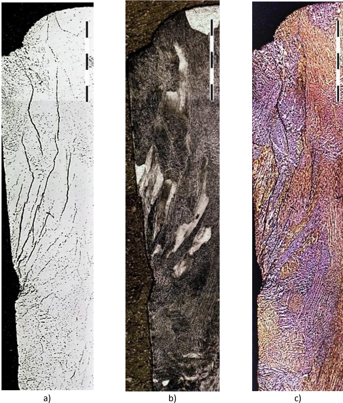
Figure 12. MIA of the affected area in: a) As polished condition, b) After etching with Poulton's etching solution, c) After etching with Wecks's etching solution
