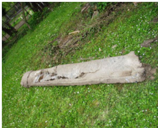
Figure 8. A piece of the remaining lead water pipe (Sisak area, Croatia), (courtesy of Ivana Miletić Čakširan)
