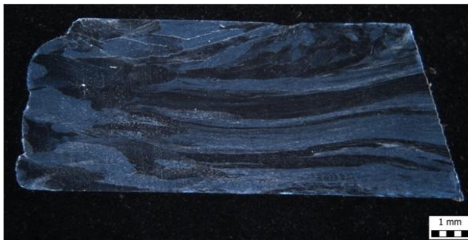
Figure 11. Macrostructure of the sample after compression testing:
