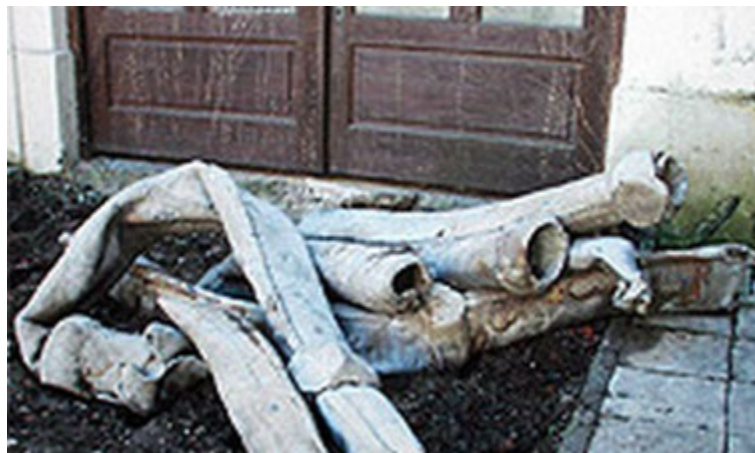
Figure 10. Roman lead water pipes after being accidentally rolled up by a dragger ship in river Kupa (Sisak area, Croatia) [20]
