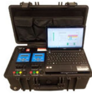
Monitoring the condition of equipment driven by an electric motor ( maintenance program on critical pumps, presses, compressors and waterjet cutters )
