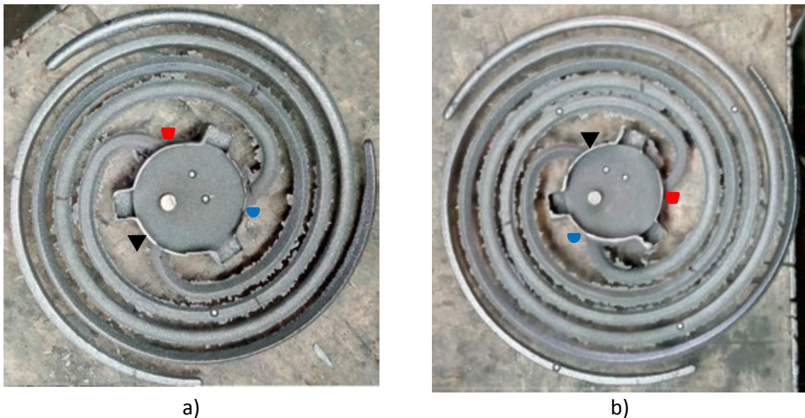
Figure 5. Measured castability at purring temperature: a) 1252 °C and b) 1311 °C
