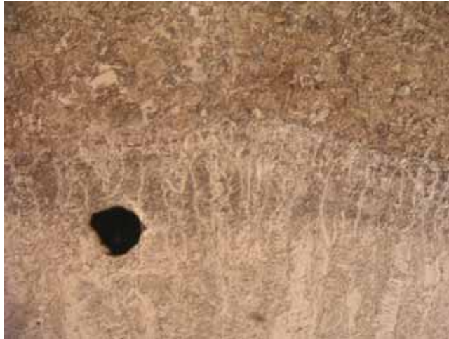
Figure 8. Inclusion in the weld metal close to the fusion line, magnification 100 x
