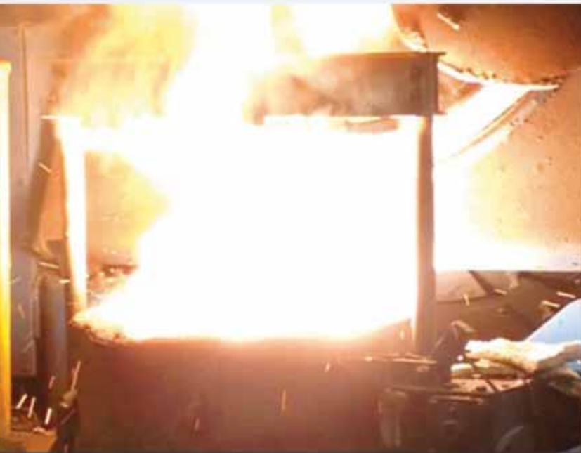
Conventional Mg Treatment with Steel cover
