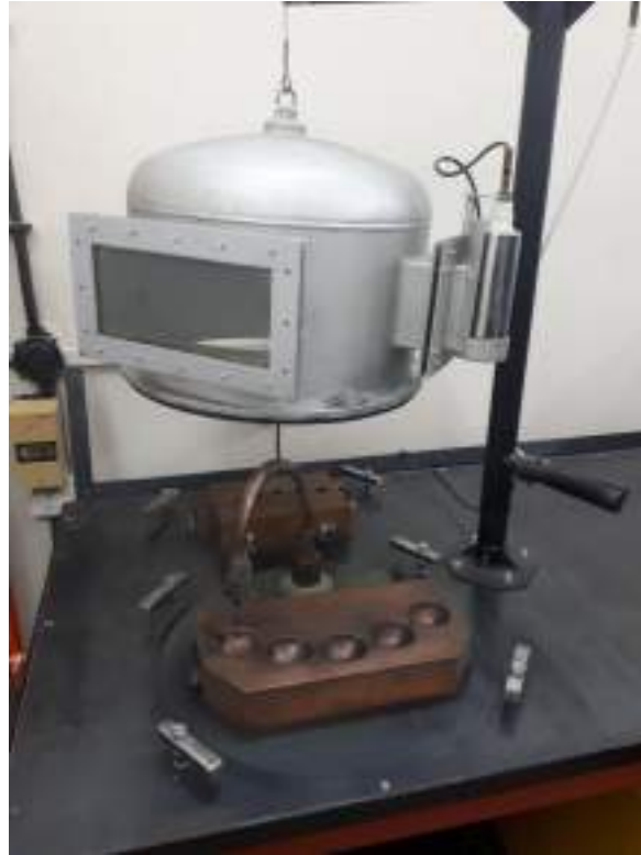
Figure 1. The laboratory electro-arc furnace used for smelting and casting in Cu-mould
