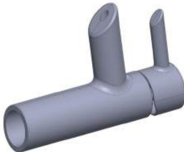
Figure 1. 3D water tap made from two parts
