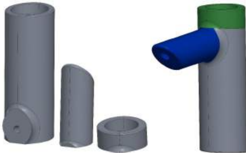
Figure 2. Water tap part 1 sliced and prepared for printing
