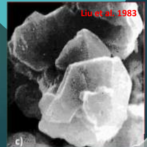
chunky graphite in cast iron
