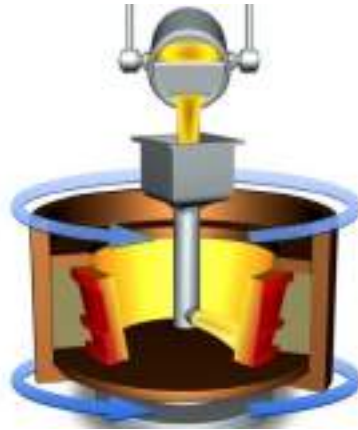
Figure 1. Vertical centrifugal casting process [8]
