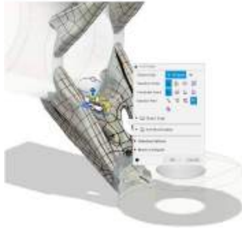
Figure 3. Editable output from GD in Fusion 360
