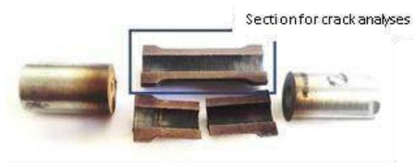
Figure 4. EDM sectioned specimen after thermal fatigue testing and a section used for further analyses
