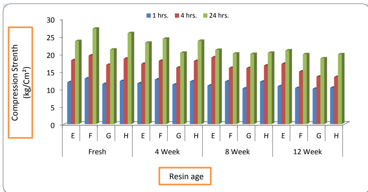
Figure 10. Hourly dry strength of samples made with fresh and aged Resin (E-H)
