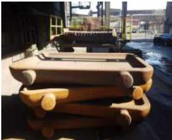
Figure 1. Ingot mold, volume V=0.25 \text{ m}^3
