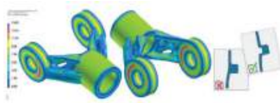
Figure 8. Visualization of design local thicknesses
