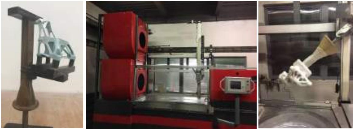
Figure 7. Preparation of the cluster and manufacture of the ceramic shell
