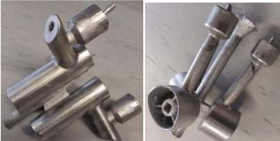
Figure 8. Casted water tap using 3D printed patterns and investment casting technology
