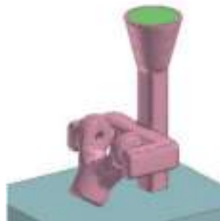
Figure 12. Shell geometry and position of the casting on the gating system
