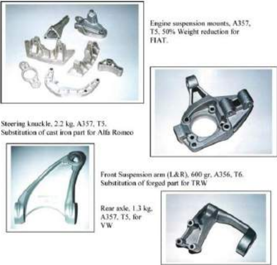
Figure 5. Parts produced by Stampal S.p.A. for various automotive manufacturers using the MHD (magneto hydrodynamic stirring) feedstock route [14]
