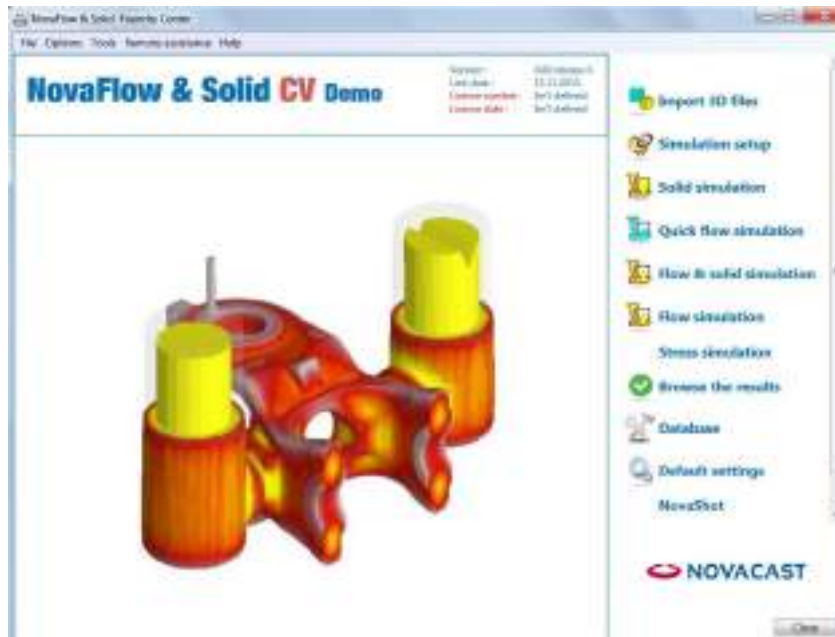
Figure 4. Interface of Demo version of simulation software NovaFlow & Solid CV Demo 4.60 r6 [12]
