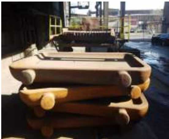
Figure 1. Ingot mold, volume V=0.25 \text{ m}^3
