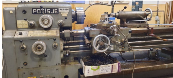
Figure 2. Conventional lathe POTISJE type ADA PA 501M
