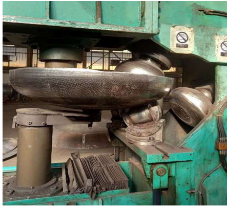
Figure 1. Production of floors by incremental deformation process [2]
