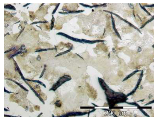
d) etched by nital 2%, magnification 200x
