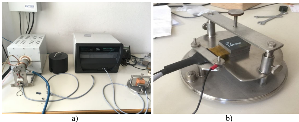
Figure 4. Instrument Hot Disk TPS 2200 (a). Measuring sensor sandwiched between two halves of a sample during measurement (b)
