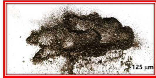
Figure 7. Titanium powder after hydrogenation and milling of TiAl6Nb7 titanium alloy
