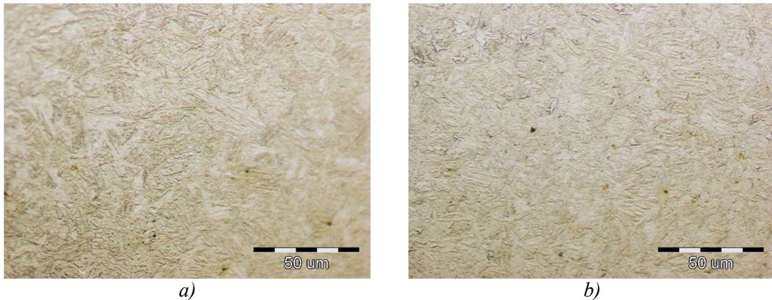
Figure 3. The microstructure of the sample cooled in the water without mixing: a) surface and b) center, x500
