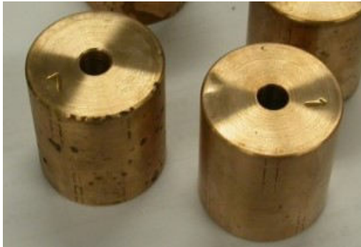
Figure 3. Disks from the ground and molded rapidly solidified Cu-Al-Ni-Mn shape memory alloy
