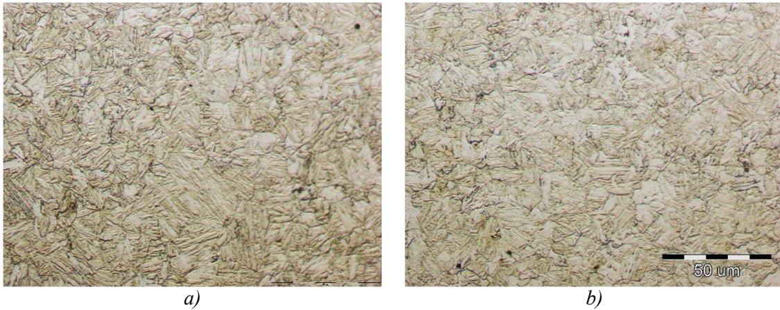
Figure 9. The microstructure of the sample cooled in the oil with a mixing of 750 rpm: a) surface and b) center, x500
