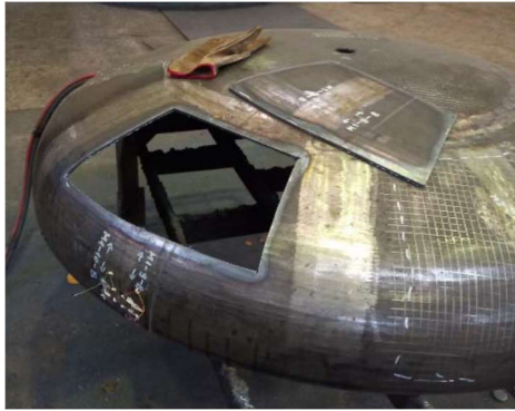
Figure 3. Taking samples from the manufactured floor
