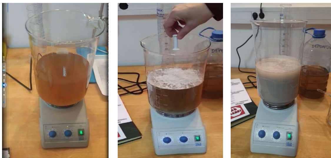
a) b) c) Figures 1. Sample of landfill leachate water before a), during b), and after c) the addition of pyrophyllite
