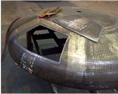
Figure 3. Taking samples from the manufactured floor
