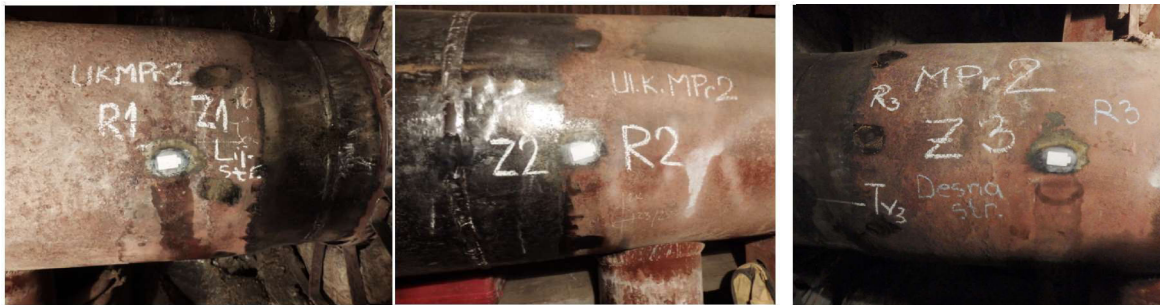
Figure 4. The position of the replicas on the header MPr 2 and photos taken from the investigated places
