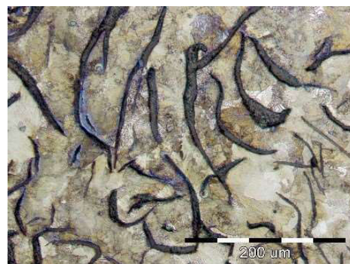
d) etched by nital 2%, magnification 200x
