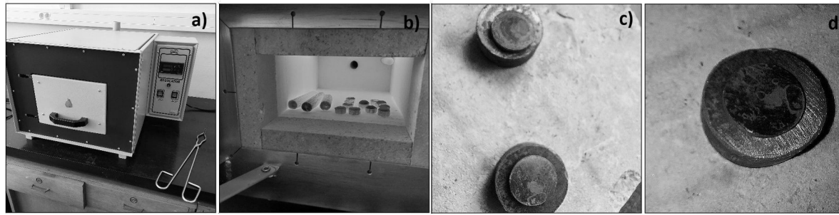
Figure 1. Equipment and different steps in the heat treatment process: a) electric resistance furnace; b) sample heating; c) and d) samples after tempering for 2 hours at different temperatures
