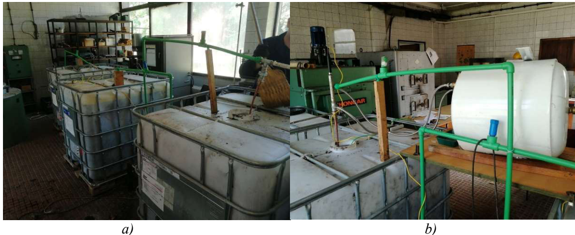
Figure 2. Controlled biodegradation system: a) Sterns in series, b) Water circulation system
