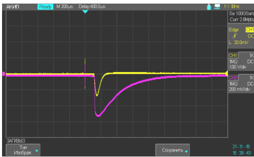
Fig. 6. Synchronous oscillograms of current pulse (CH1) and the radiation (CH2) of the electropulse discharge in water (capacitive energy storage voltage U_{max} = 1.5 kV).
