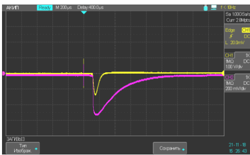
Fig. 6. Synchronous oscillograms of current pulse (CH1) and the radiation (CH2) of the electropulse discharge in water (capacitive energy storage voltage U_{max} = 1.5 kV).
