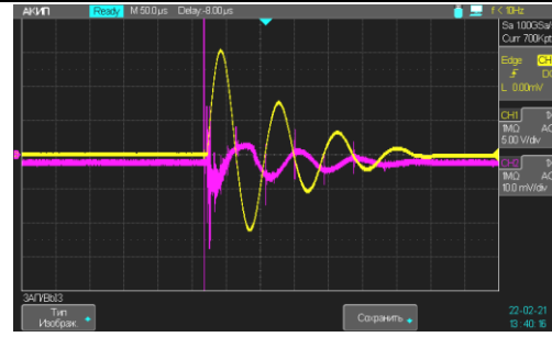
Fig. 4. Synchronous oscillograms of current pulses (CH1) and the radiation of a powder material (CH2) during consolidation process (capacitive energy storage voltage U_{max} = 3 kV).
