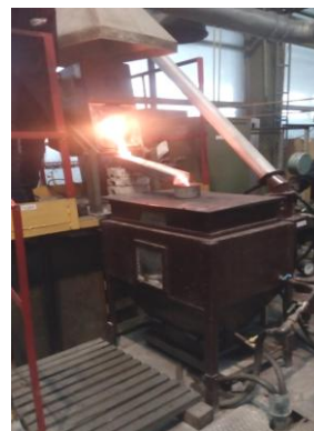
Fig. 2. The process of spraying copper-based powders
