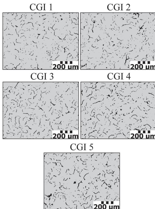
Figure 1 Graphite structure in examined CGI samples
