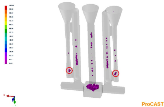
(e) Casting porosity ratio
