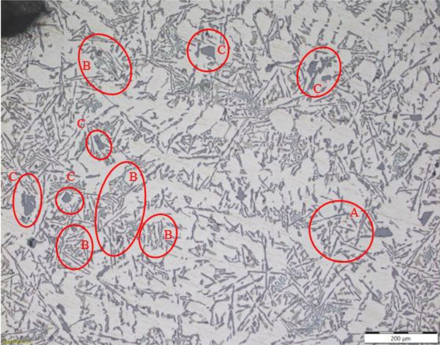
Figure 6. Al alloy AlSi_9Cu_3(Fe) at magnification 200x
