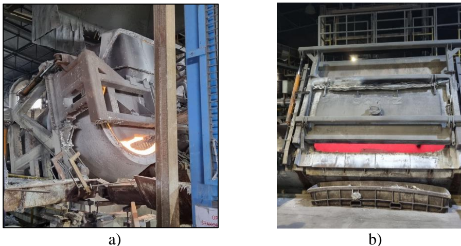
Figure 3. a) Tilting rotary furnace, b) Furnace for alloying and maintaining the melt
