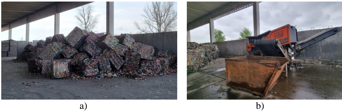
Figure 2. a) Compressed returnable packaging b) Shredder with magnetic separator
