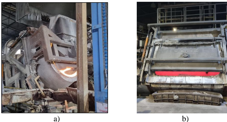
Figure 3. a) Tilting rotary furnace, b) Furnace for alloying and maintaining the melt
