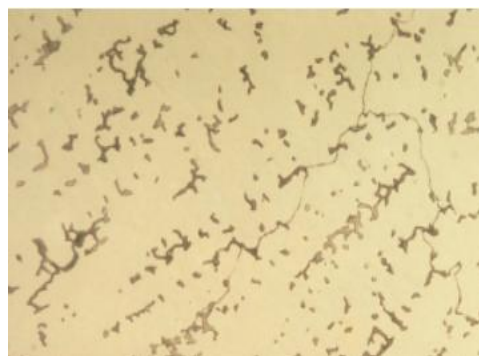
Figure 2. Microstructure of as cast and wrought Co-Cr-Mo alloy, 200x [11]
