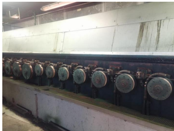
Figure 4. Machines for continuous wire drawing
