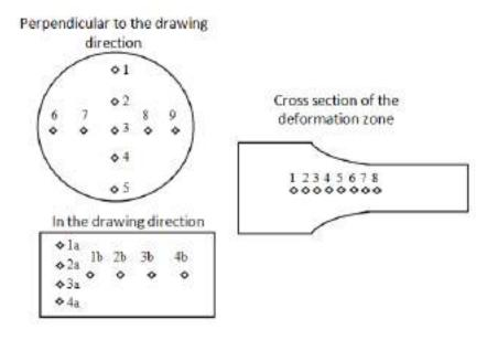
Figure 1. Scheme of hardness measurement on the samples
