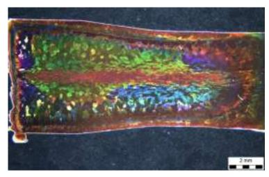
Figure 6. Macrostructure of the deformation zone during second pass
