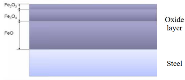
Figure 4. Oxide layer on strip surface [2]
