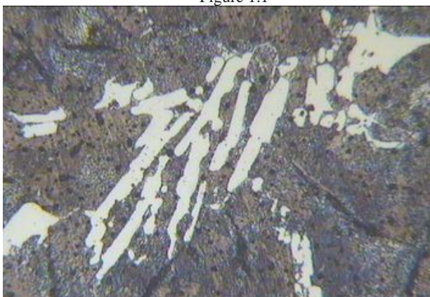
x200- Metal base + carbides + graphite plate Figure 1.2
