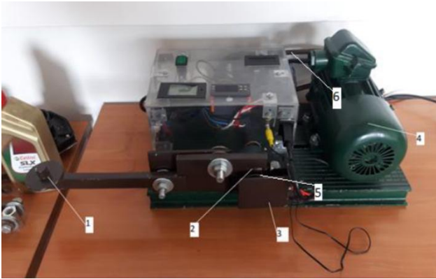
Fig. 1. The Timken test experimental setup: 1 – lever with the load, 2 – sample, 3 – oil bath, 4 – electric motor, 5 – shaft
