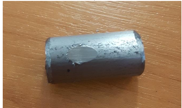
Fig. 3. Timken sample after 7 minutes of abrasion
