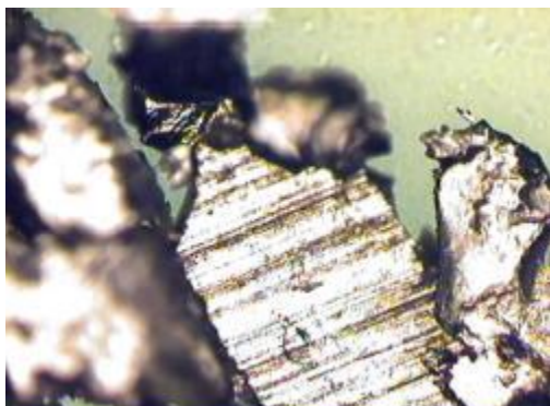
Fig. 6. Abrasion particle surface profile (1000x) [10]
