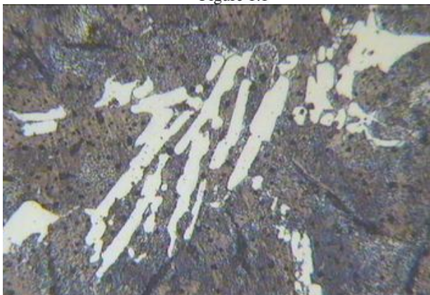
x200- Metal base + carbides + graphite plate Figure 1.2
