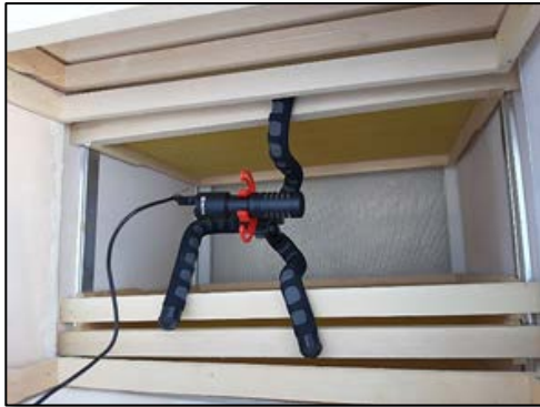
Fig. 2. Installation of the microphone inside the beehive
