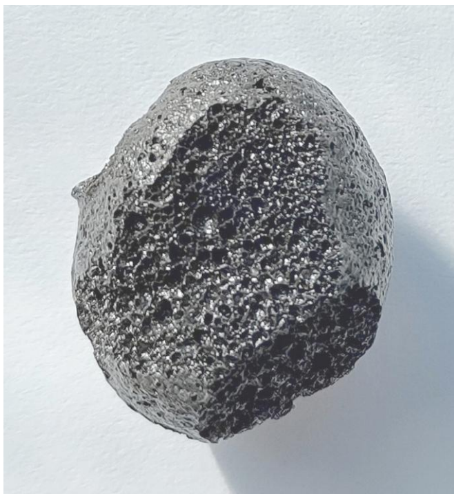
Fig. 3. Foam silicate specimen (horizontal and side section).
