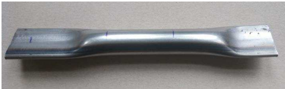
Figure 2. Samples for static tensile testing
