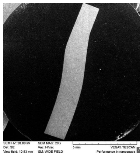
Figure 4. Sample put into the conductive mass for metallographic analysis
