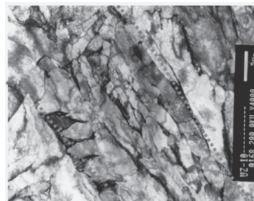
Figure 2 The orientation of grains after rolling of steel
