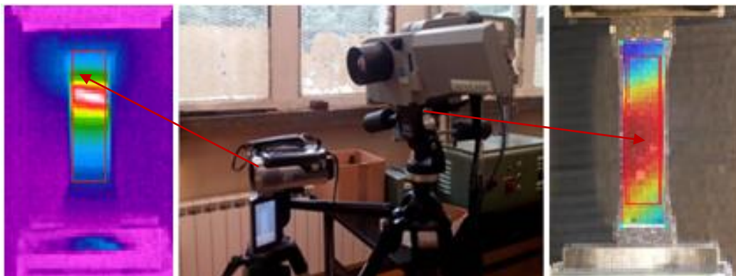
Figure 1. The arrangement of the measuring equipment as well as the deformation zone analyzed by the thermography and DIC methods
