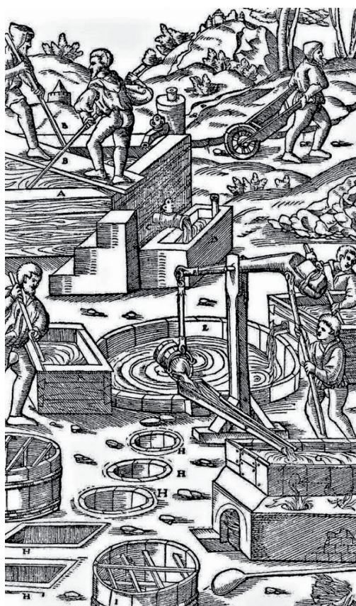
A – tanks, B – stirring poles, C – plug, D – trough, E – reservoir, F – launder, G – lead cauldron, H – wooden tubs sunk into the earth, I – vats in which twigs are fixed
