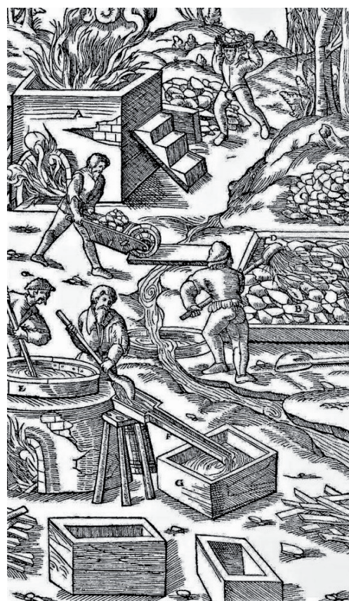
A – furnace, B – enclosed space, C – aluminous rock, D – deep ladle, E – caldron, F – launder, G - troughs
