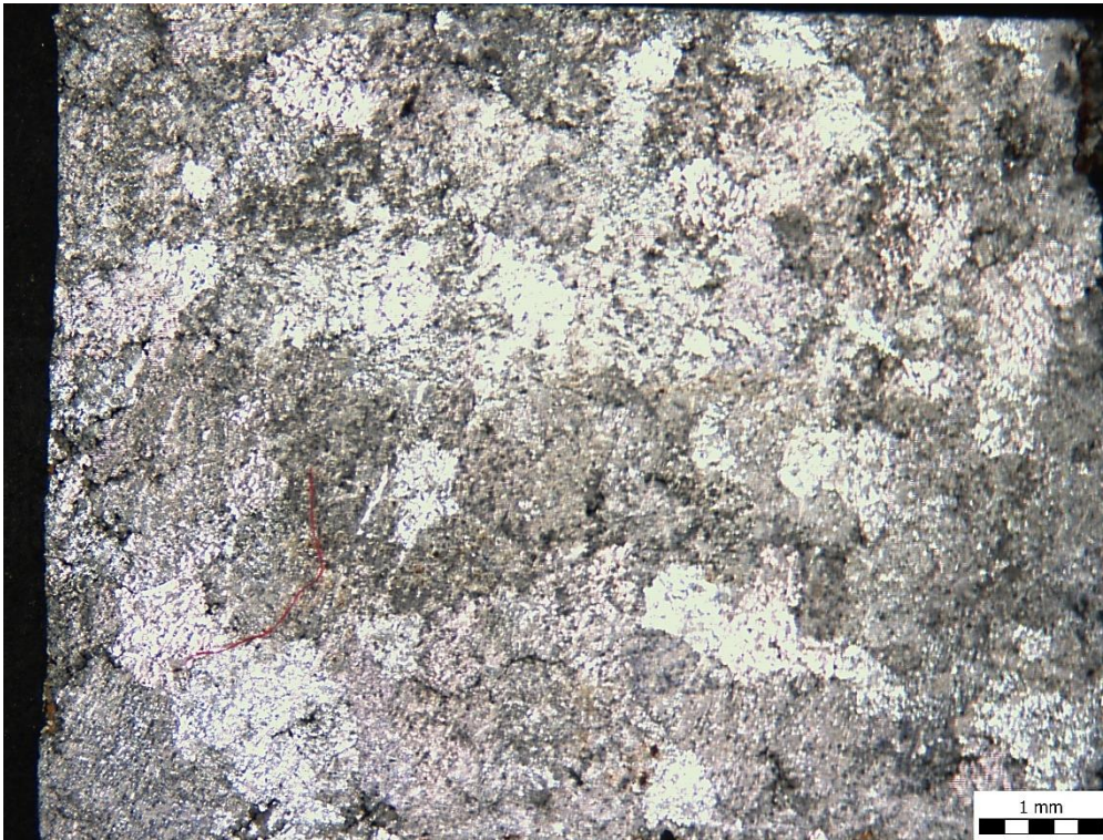
Macrostructure of the exposed surface of sample TO1 at a magnification of 17.5 X
