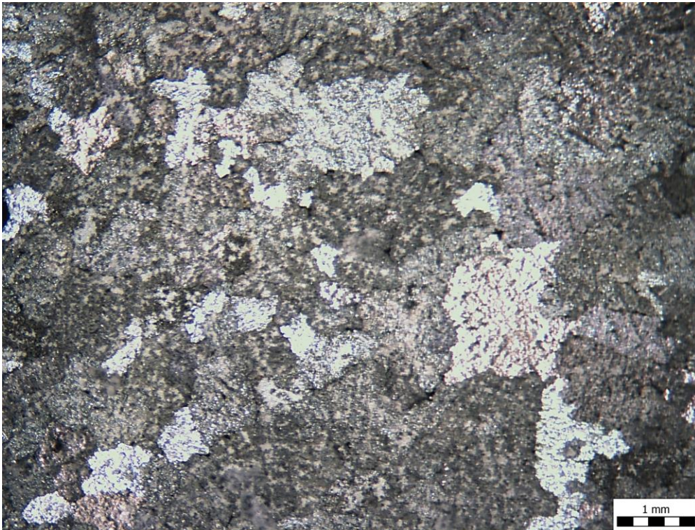
Macrostructure of the exposed surface of sample AC2 at a magnification of 17.5 X
