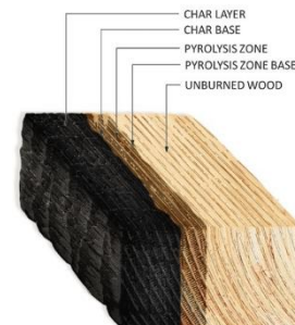
Figure 1. Superficial carbonization structure of wood exposed to the fire [5].
