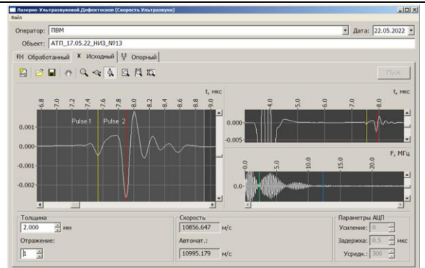
Figure 4. Screenshot of the UDL-2M screen. Testing a sample PDC with a bad interface.
