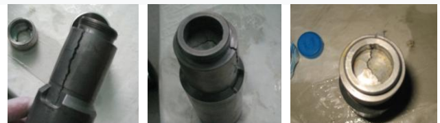
Fig. 6. Crack on the body of the source holder.
