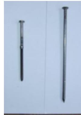
Fig. 3. Comparison of the ordinary and the new nails: a – comparison of the cross-section dimensions; b - view of the used nails with the new shape and φ7
