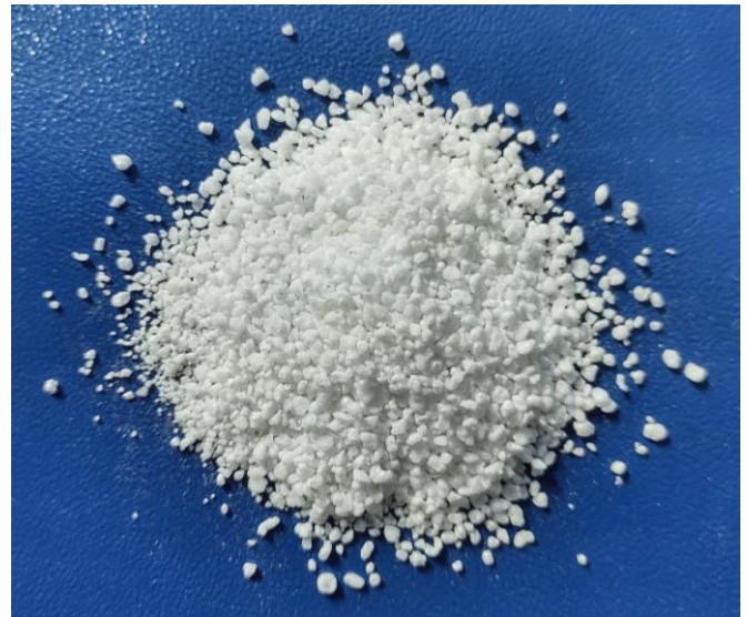
Fig. 1. Perlite for construction (fraction up to 3 mm).
