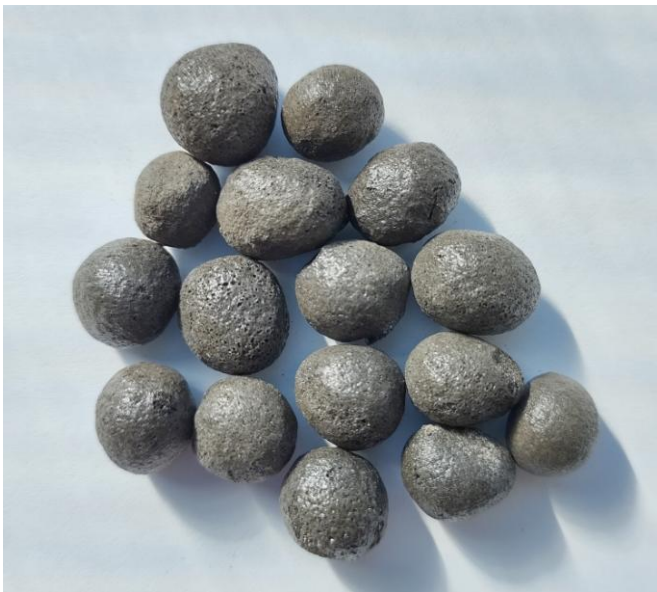
Fig. 2. Foam silicate specimens obtained from foamed waste glass.
