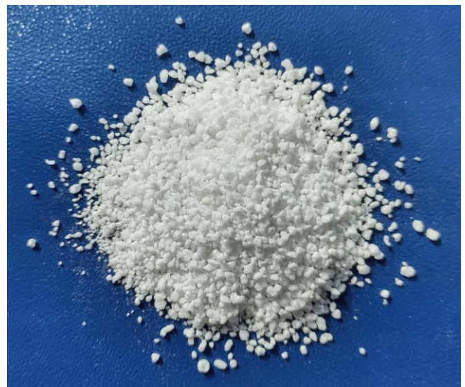
Fig. 1. Perlite for construction (fraction up to 3 mm).
