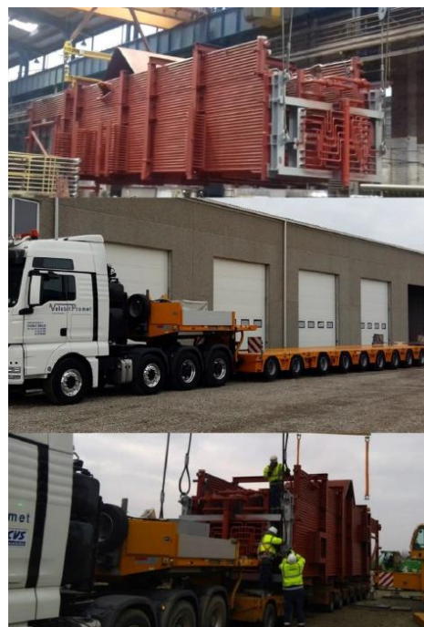
Fig. 1 Steam boiler module transport
