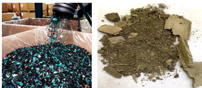
Fig. 1 Main components of polymer - mineral composition; recycled polymer plastic and mineral waste, example
