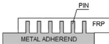
Fig. 7 Schematic of an advanced hybrid metal/composite pin joint. The pin joints combine adhesive bonding with mechanical interlocking [6]
