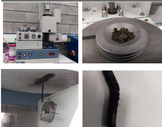
Fig. 6 View of MFI instrument, Ceast 6542.0 and selected measurement samples.
