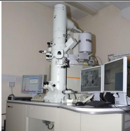
Fig. 1. Multipurpose transmission electron microscope JEOL JEM 2100.
