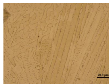
Fig. 8 Microstructure of cover layer clad with UTP A 702
