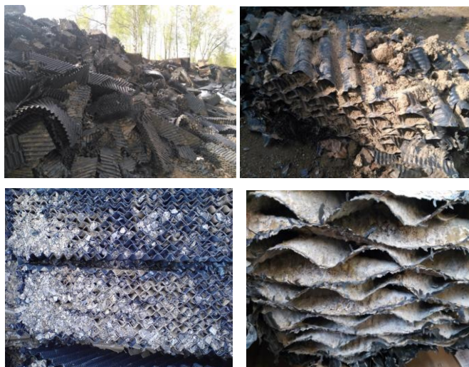
Fig. 2 View of used cooling tower sprinklers used in processability studies of polymer - mineral composites.
