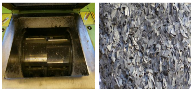
Fig. 3 The appearance of the shredder blades and the made polymer-mineral recyclate.
