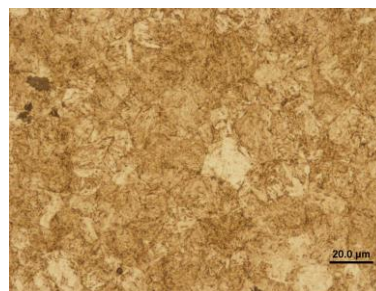
Fig. 5 Microstructure of base material (BM) Dievar
