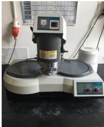
Slika 34. PHOENIX BETA GRINDING/POLISHER s glavom Vector LC
