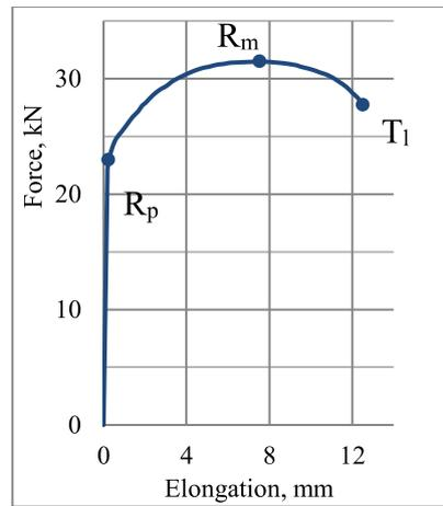
**Fig. 3: Diagram obtained by static tensile test**
