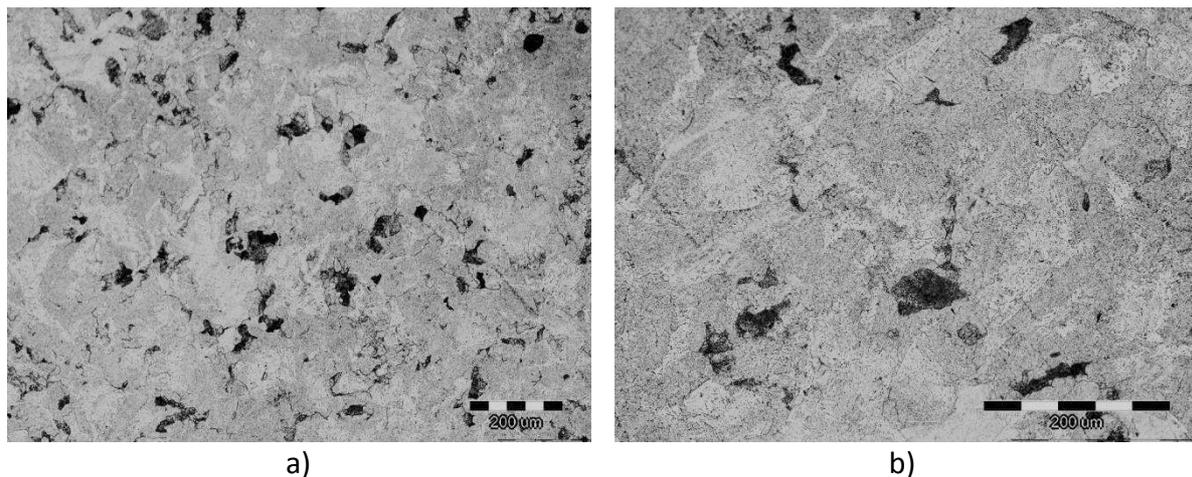
Figure 4. Microstructure of HTCS-130 tool steel for hot work after etching in Nital:
