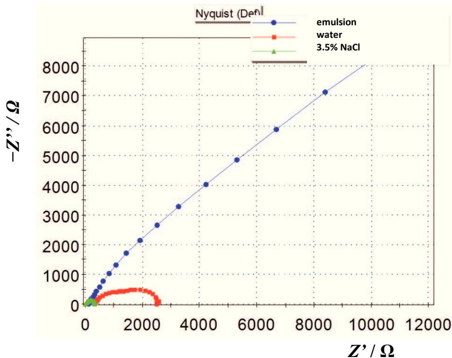
Figure 2. The comparative view of Nyquist's EIS diagrams obtained for HCTS-130 tool steel in medium of Lenox Band-Ade emulsion, water and 3.5% NaCl
