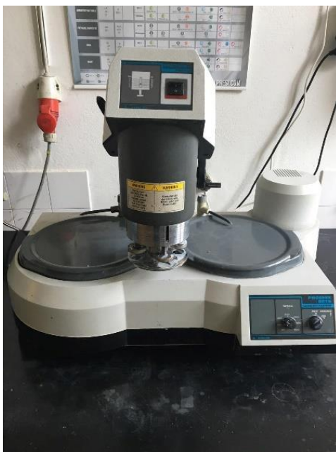
Slika 26. Uređaj PHOENIX BETA GRINDING/POLISHER s glavom Vector LC
