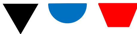
Figure 2. Cross-section shape of gating system for spiral probe – all have cross-section area 40 \text{ mm}^2 [3]
