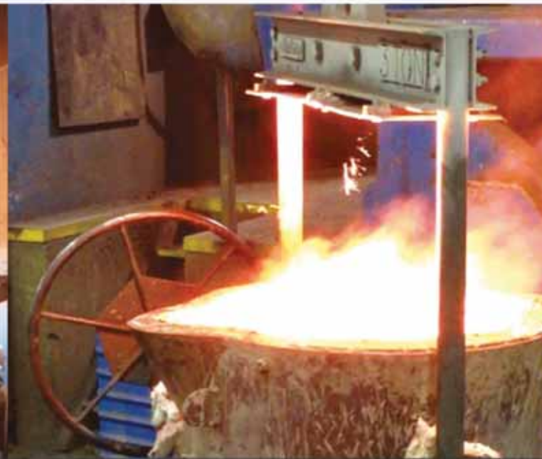
Improved Mg Treatment with TOPSEED* cover alloy
