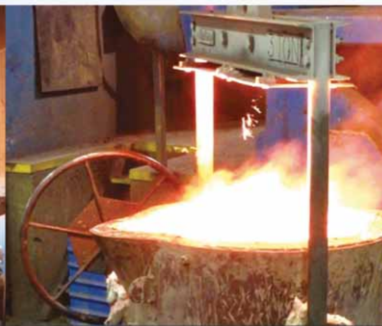
Improved Mg Treatment with TOPSEED* cover alloy
