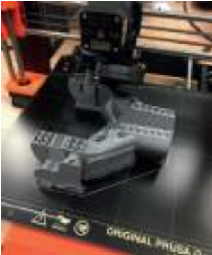
Figure 14. 3D printing of model from PLA material
