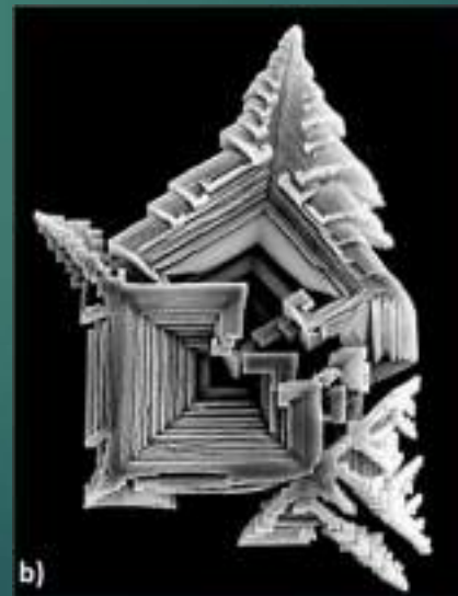
dendritic/hopper crystal in salt
