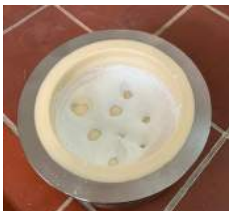
Figure 1. 70 wt% of dry alumina water-based suspension after homogenization
