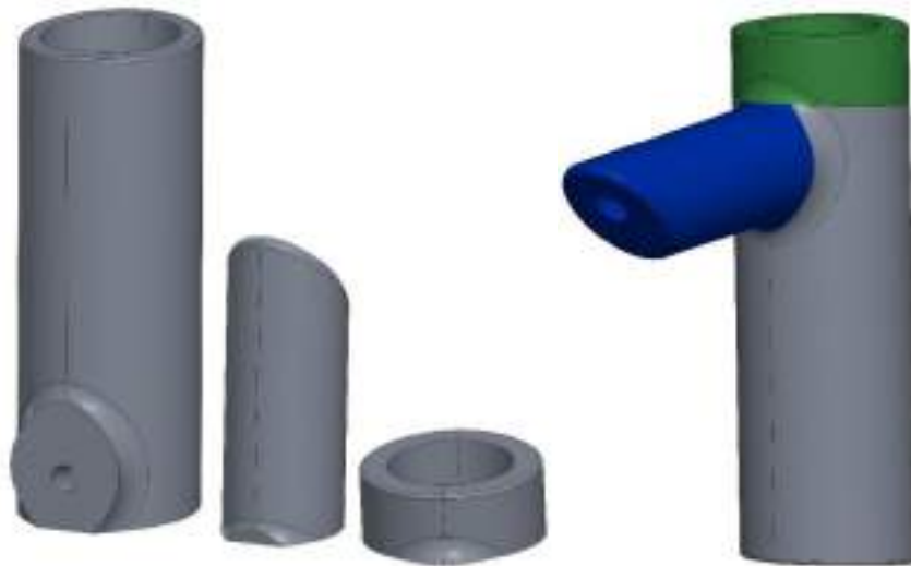
Figure 2. Water tap part 1 sliced and prepared for printing
