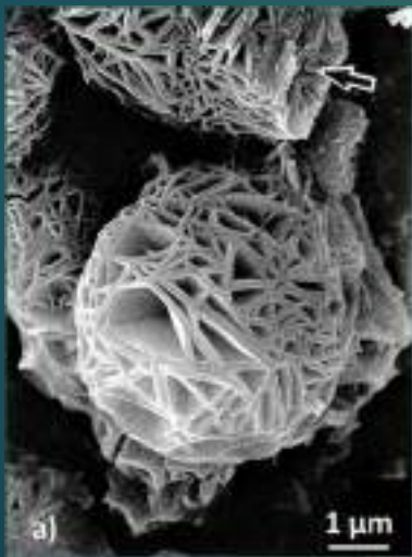
hopper crystal in a \beta - \text{Si}_3\text{N}_4 crystal
