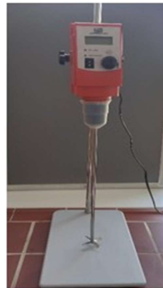
Figure 1. Digital overhead Stirrer LLG-uni STIRRER OH2
