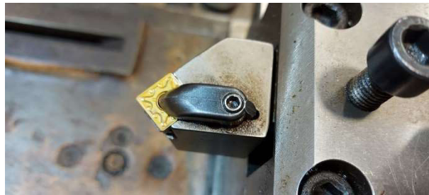
Figure 4. Replaceable cutting insert type SNMG 120408-MAUS735
