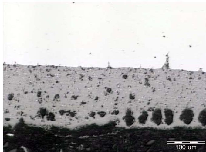
Figure 2. The oxide layer, inside the wall of the pipe [8]
