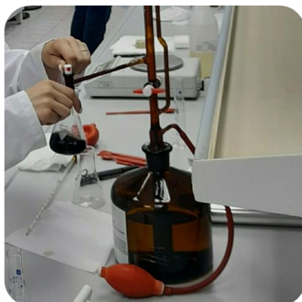
Slika 3. Određivanje Pbr po Wheeleru (izvor autor) Figure 3. Determination of Pbr according to Wheeler (source author)
