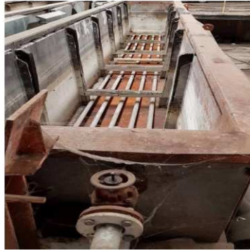
Figure 3. Tub with heaters [7]
