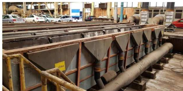
Figure 2. Tubs for tube preparation [7]
