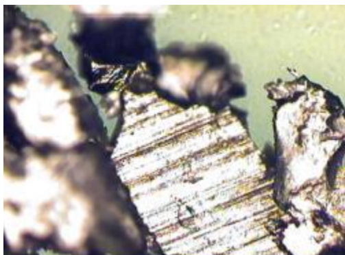
Fig. 6. Abrasion particle surface profile (1000x) [10]
