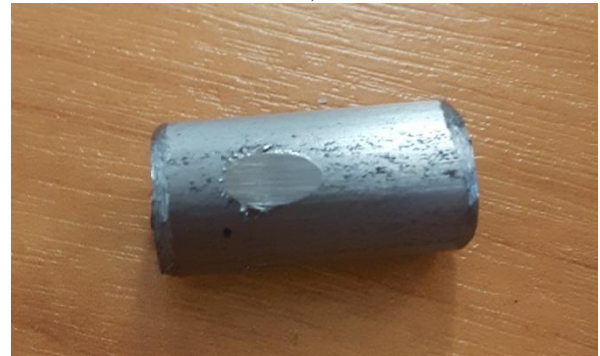
Fig. 3. Timken sample after 7 minutes of abrasion
