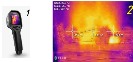
Fig.6. Temperature measurement remotely: 1 – thermal imager FLIR TG297 [15], 2 – an image with measuring results.
