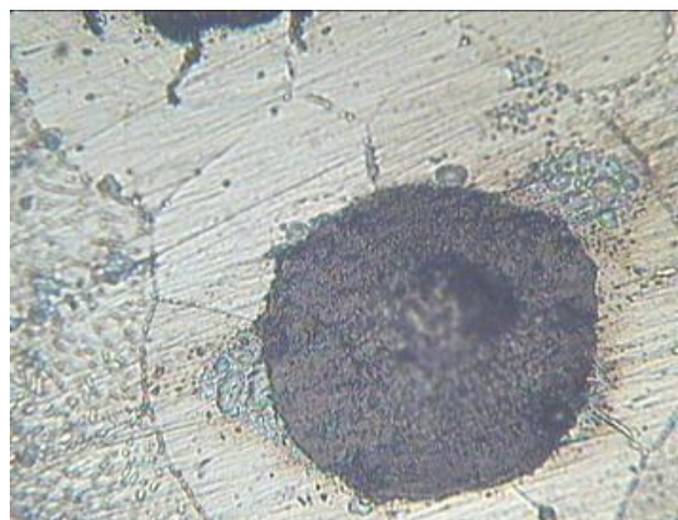
x500- Metal base (perlite) + spheroidal graphite + ferrite Figure 2.7
