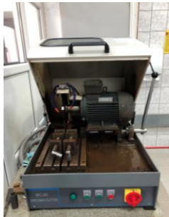
Fig. 1 Device for cutting specimens.
