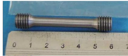
Fig. 4. Specimens for tensile testing
