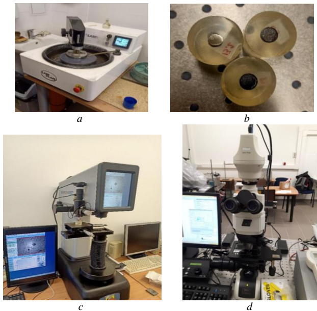
Fig. 1. Experimental setup: grinding of samples with Lamplan machine, b – prepared samples, c - the Innova test machine for determining hardness value, d – examination of the structure using optical microscope Nikon
