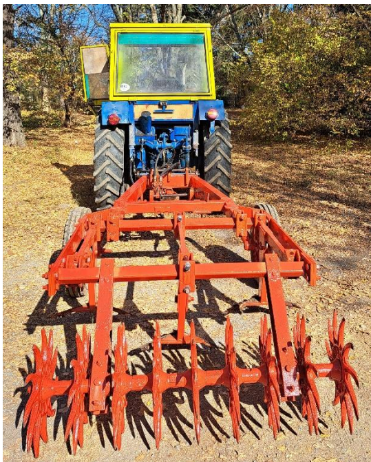
Fig.2. Trial model of combined machine for inter-row cultivation of perennial crops, rear view
