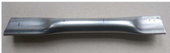
Figure 2. Samples for static tensile testing
