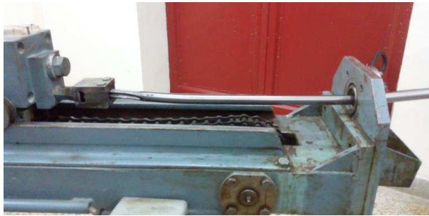
Figure 1. Drawing of tube on the laboratory drawing bench
