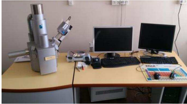
Figure 5. Scanning electron microscope Tescan Vega 5136mm
